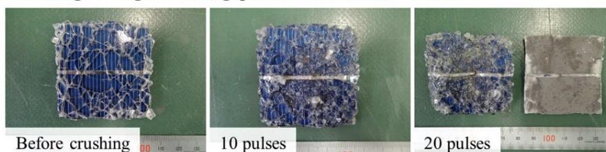
Discharge voltage: 130 kV, gap between electrode: 20 mm
