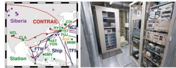
Figure 2. (left) Map showing the locations of atmospheric GHG observations in the Asia-Pacific region. Green circles represent ground site locations, blue lines indicate ship routes, and red lines indicate aircraft flight routes. (right) Photograph showing atmospheric observation systems at a broadcasting tower (Tokyo Skytree).
