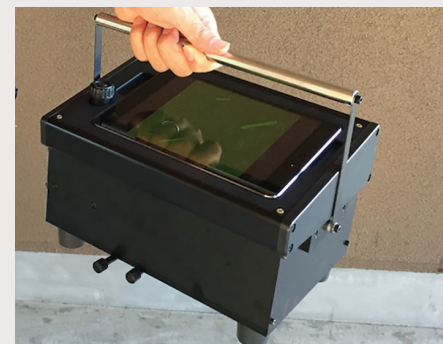
A robust and portable fluorescence microscope has been developed for the on-site asbestos detection. Magnification (approximately \times 300 ) can be digitally increased (until \times 1,000 ).
